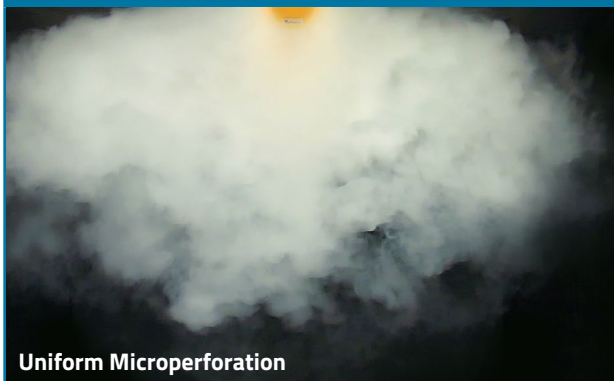
Examples of airflow patterns created using smoke tests in the PRIHODA R&D centre
