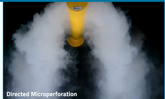
Examples of airflow patterns created using smoke tests in the PRIHODA R&D centre
