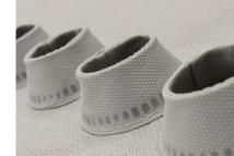
Fabric pockets are used for aligning deflection of the air coming from the perforation. The solution is based on combining two airflows of a similar momentum. The flow from the last hole in the row is directed under a certain angle using a fabric pocket, thus aligning the air deflection from the perforation.
