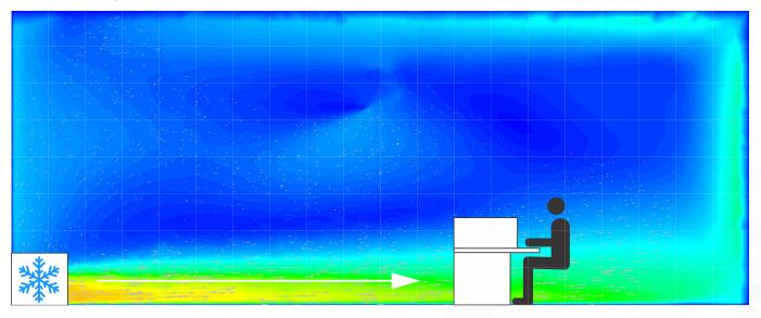
Example: cold air from the freezing counter makes the work of the cash register operators uncomfortable.
