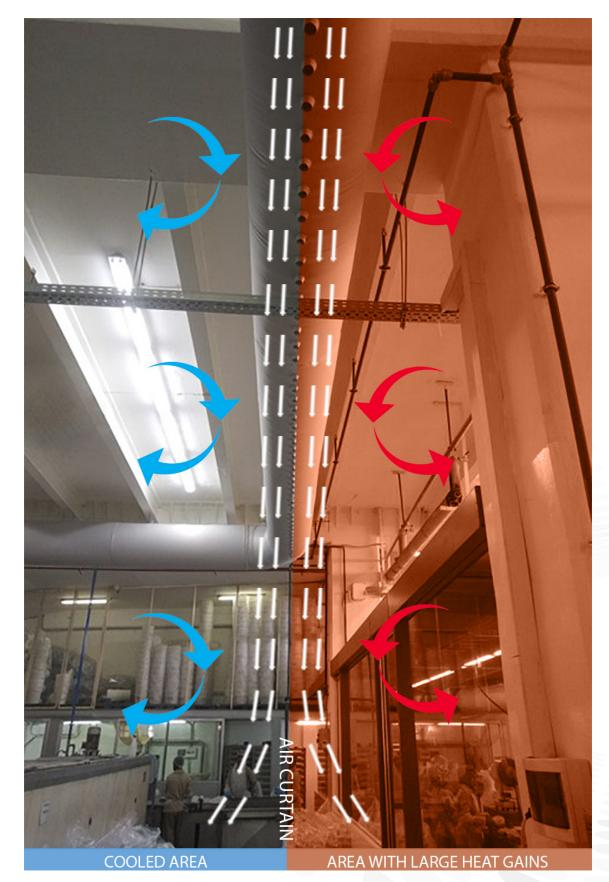
The heat generated by the furnaces in the production sector is diverted and does not enter the sector designated for product packaging.
